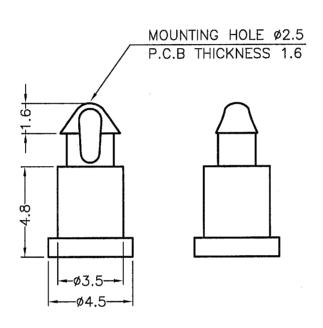
NOTE: All measurement does not include gate which raises under 0.3mm.
